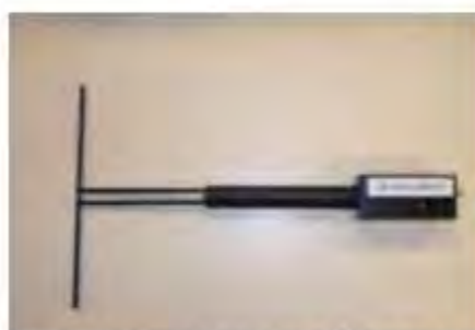
Figure 1 – Satimo COMOSAR Validation Dipole
