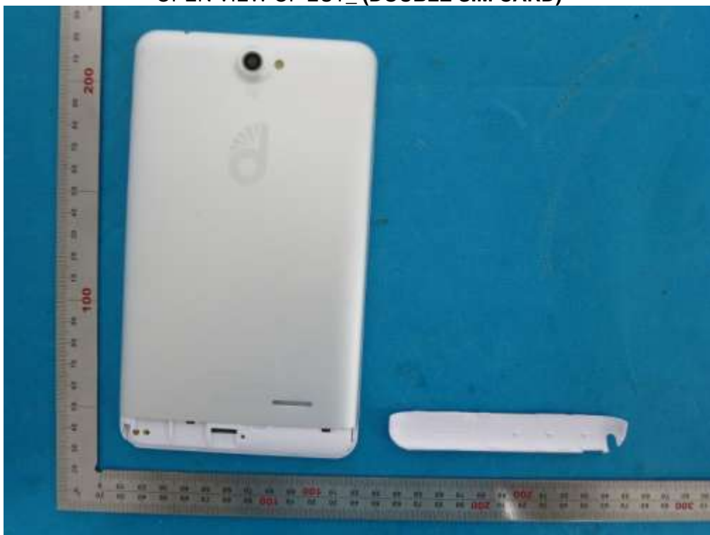
OPEN VIEW OF EUT_ (DOUBLE SIM CARD)
