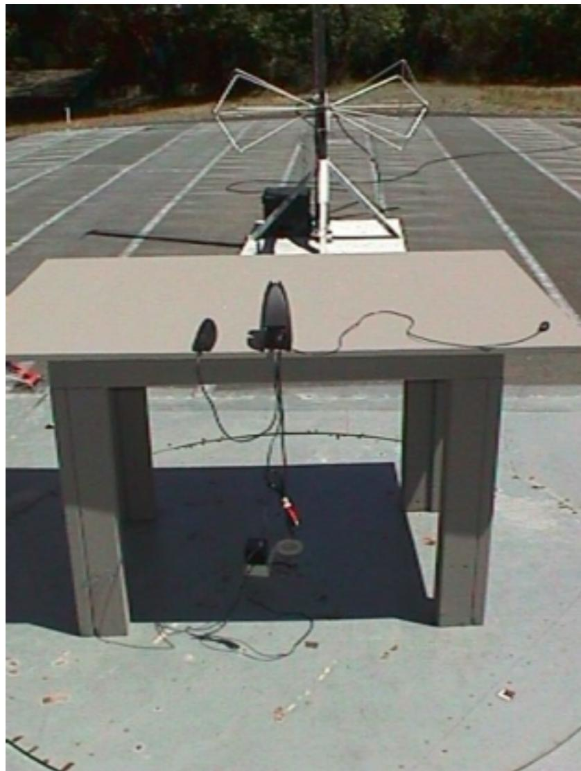
**Front View of the Base Station EUT for Intentional Radiator Emissions Tests**
