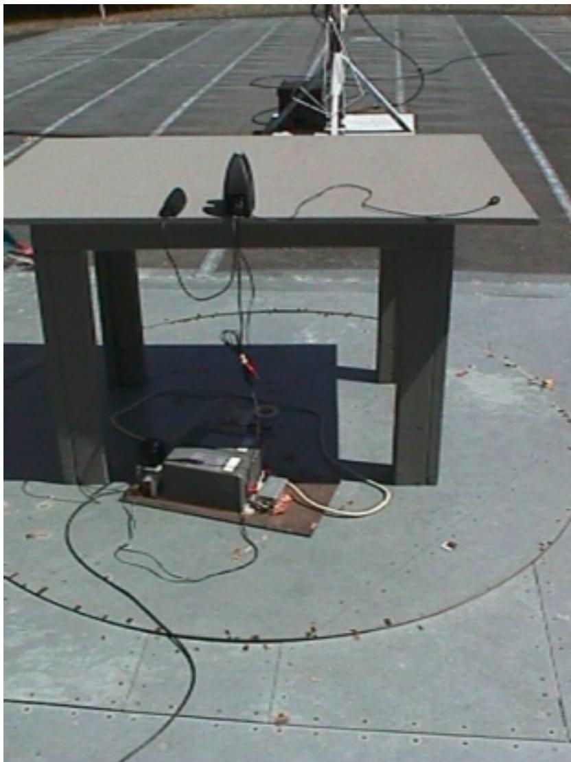
**Front View of the Base Station EUT for Unintentional Radiated Emissions Tests**
