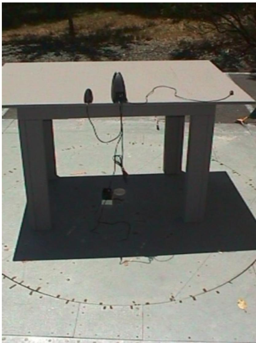
**Rear View of the Base Station for Unintentional Radiated Emissions Tests**
