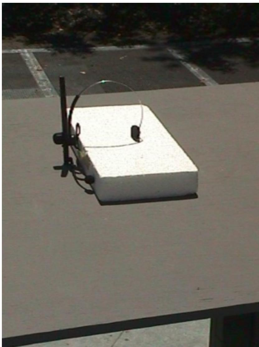
**Rear View of the Headset EUT for Intentional Radiator and Unintentional Radiated Emissions Tests**
