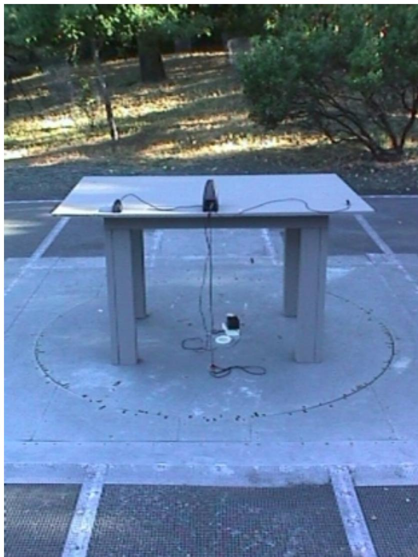
**Rear View of the Base Station EUT Intentional Radiator Emissions Tests**
