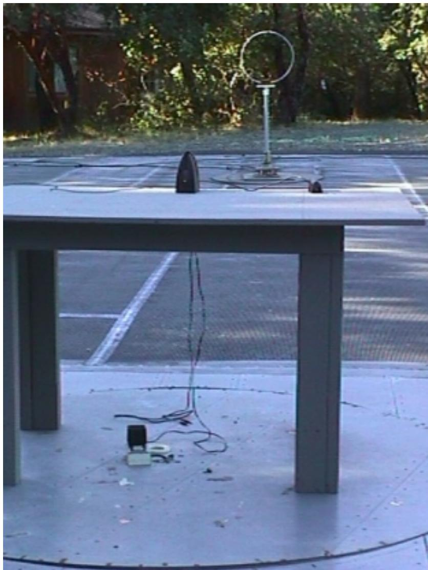
**Front View of the Headset EUT for Intentional Radiator and Unintentional Radiated Emissions Tests**
