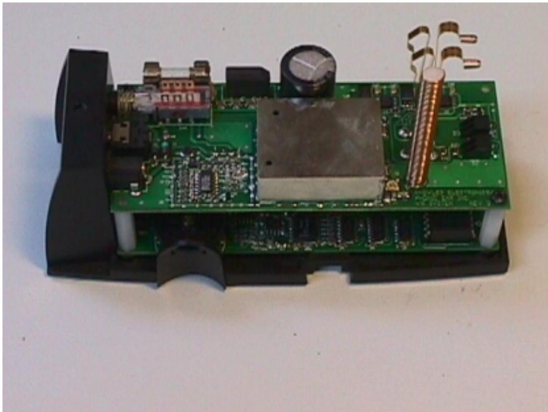
**Views of the Front and Back Side of the Magnetic Transmitter PC Board**
