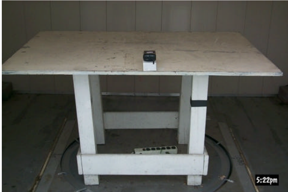
Figure 3.1 Radiated Test Setup, X-Axis
