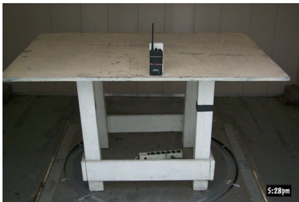
Figure 3.3 Radiated Test Setup, Z-Axis
