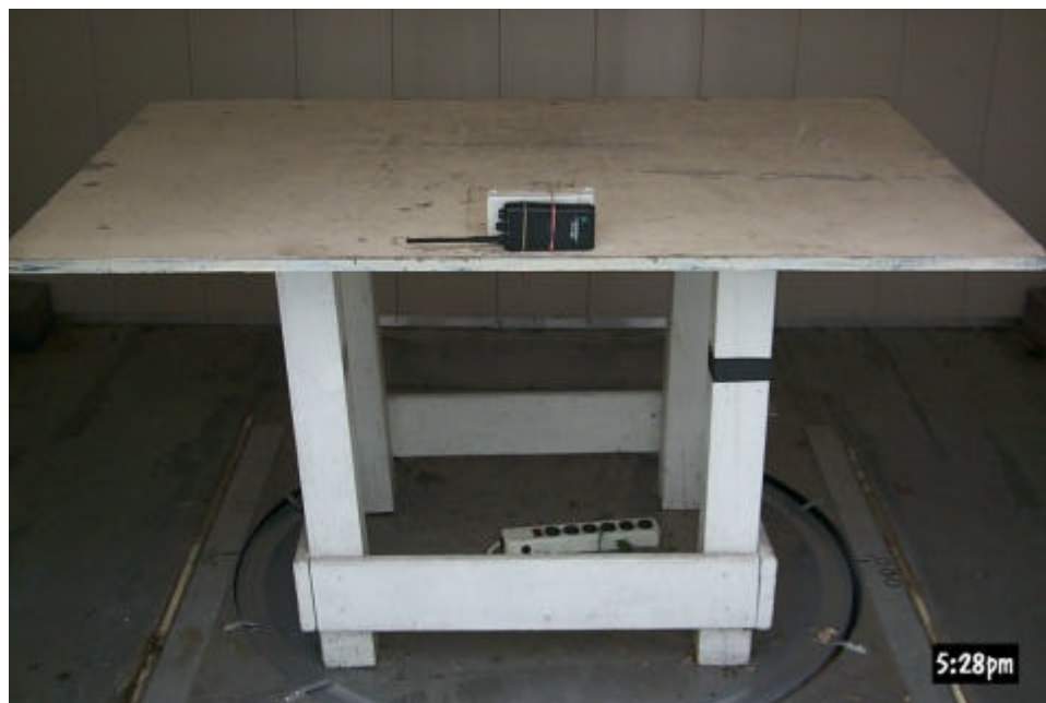
Figure 3.2 Radiated Test Setup, Y-Axis
