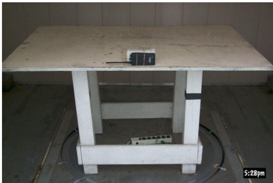
Figure 3.2 Radiated Test Setup, Y-Axis
