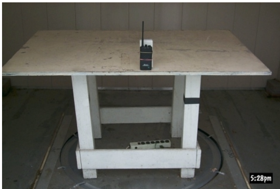
Figure 3.3 Radiated Test Setup, Z-Axis
