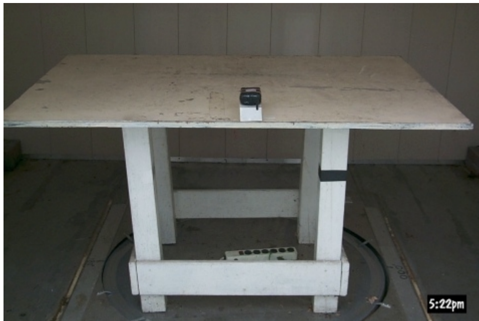
Figure 3.1 Radiated Test Setup, X-Axis
