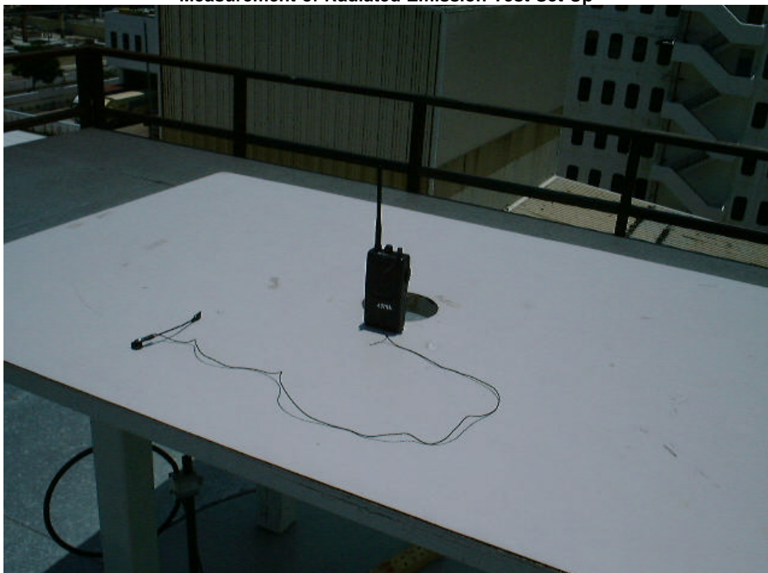
Measurement of Radiated Emission Test Set Up
