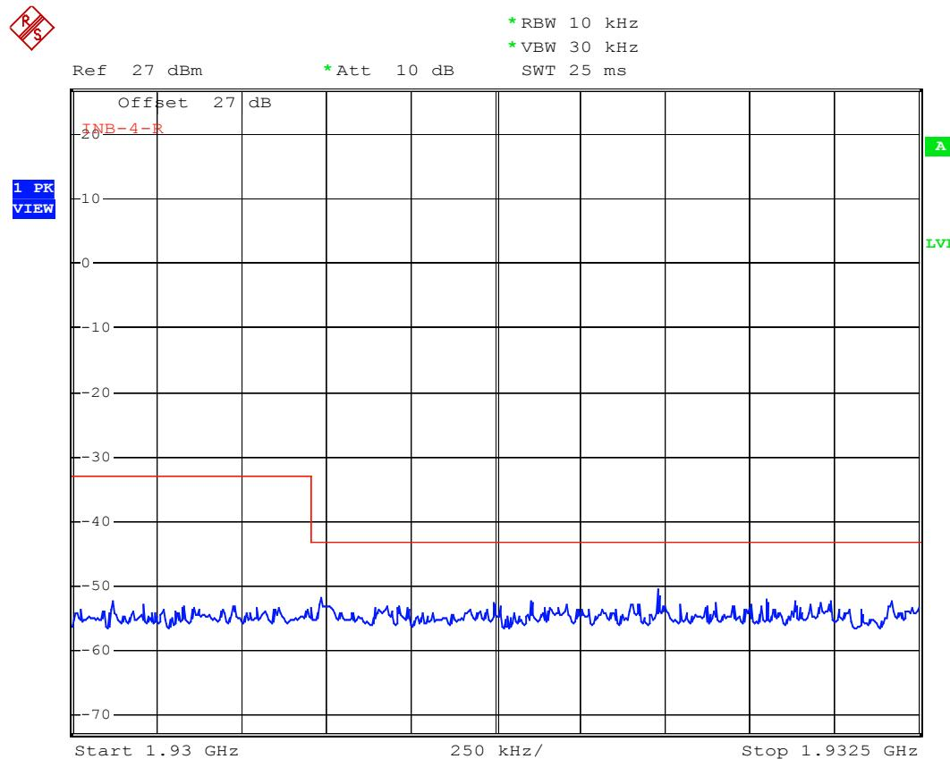
b) CH F<sub>H</sub>Out-of -band Unwanted Emission (above 1GHz): CH F<sub>H</sub>Operation Mode : TransmittingFundamental Frequency : 1928.450MHzTest Date : Jan. 19, 2009 Temperature : 20 °C Humidity : 58 %
