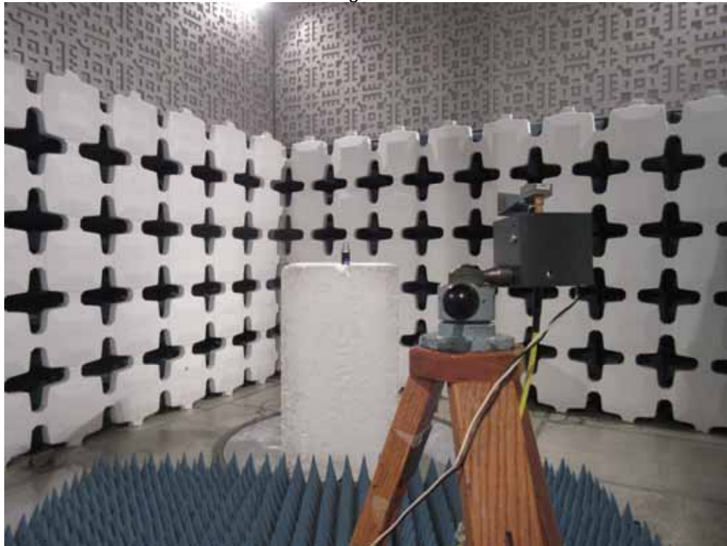
Test Setup for Radiated Emissions – 18GHz to 25GHz, Horizontal Polarization
