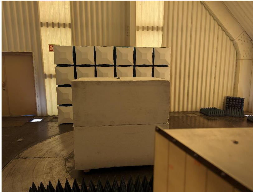
Photograph 3: Front View Radiated Emissions Worst-Case Configuration – Above 1000 MHz
