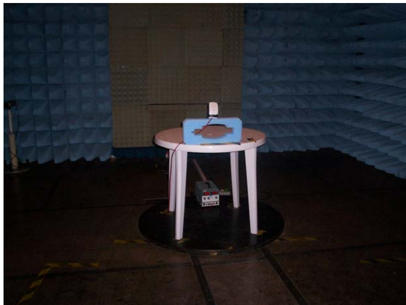
Radiated Emissions (Tested by RN Electronics Ltd)
