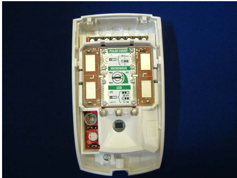
EUT (Front Face Removed – Exploiting Microwave Module)
