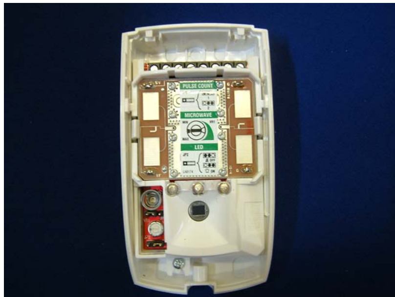
EUT (Front Face Removed – Exploiting Microwave Module)
