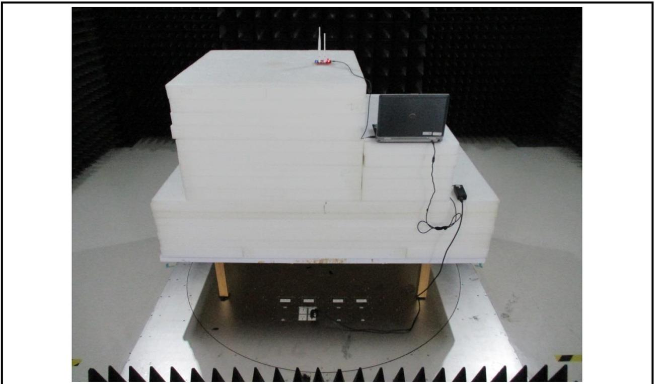
Radiated Emission Above 1GHz Test
