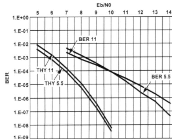
FIGURE 15. BER vs Eb/N0 PERFORMANCE FOR CCK MODES
