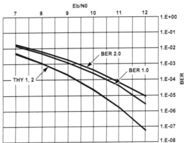
FIGURE 14. BER vs Eb/N0 PERFORMANCE FOR PSK MODES
