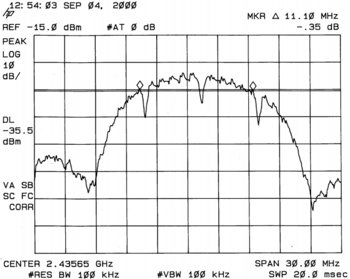
Plot 1.2: -6 dB bandwidth plot of channel 6 at 2.0 Mbps
