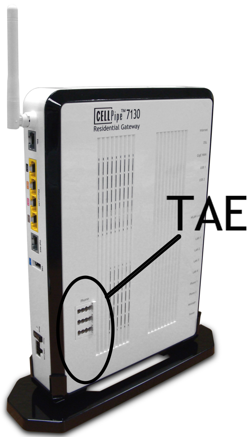
Figure 1-4 TAE interface for the CellPipe 7130 6Ve.B2131 residential gateway
