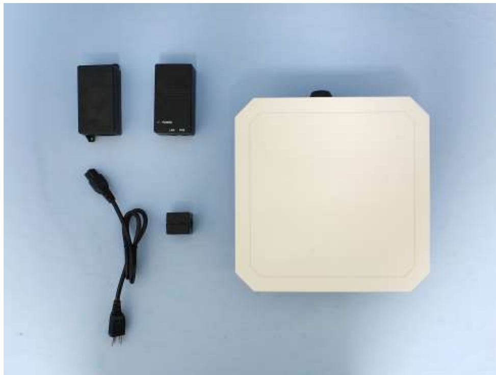
Antenna with 15.43dBi gain
