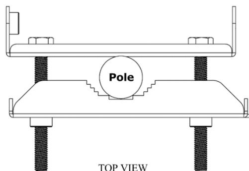
3. With the connector facing downward, and assembling two brackets together. Thread the M10\*20mm bolt through a spring washer, flat washer and the bracket holes.
