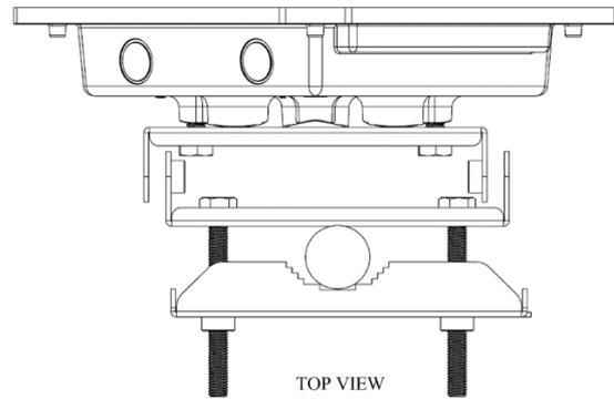
4. Adjust the required angle and lock the screws. This is an angle that can be adjusted 10 degrees above and below.
