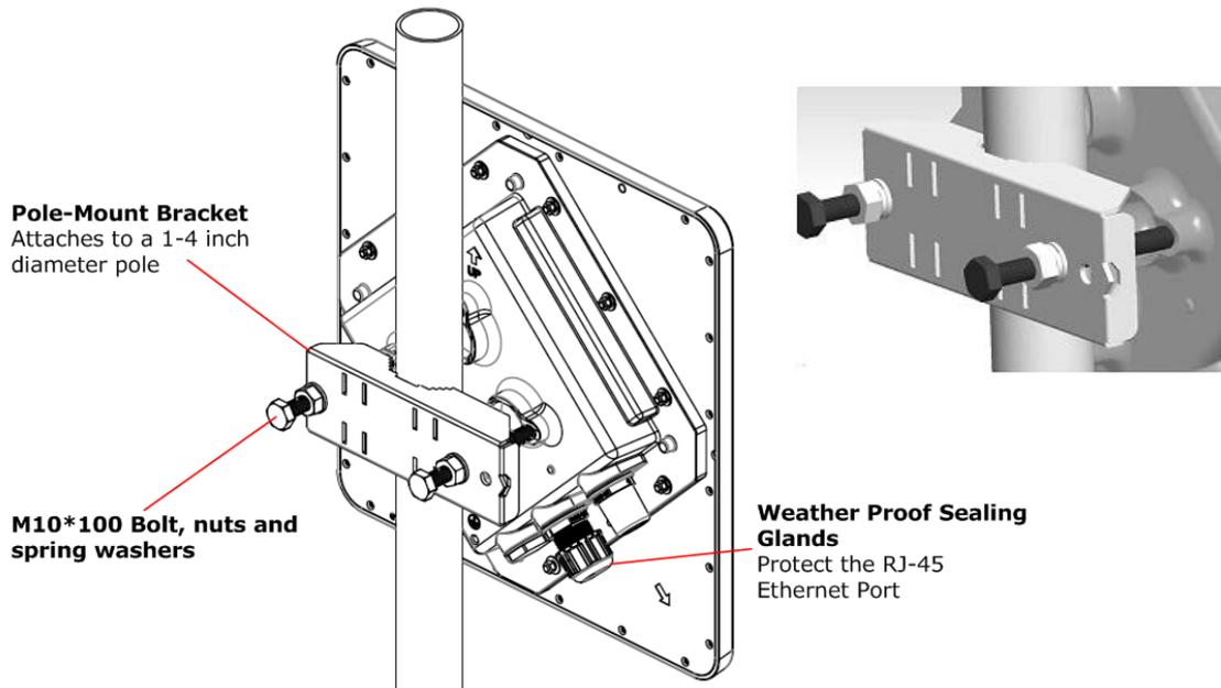
• **Using the clamp [adjustable angle]**
