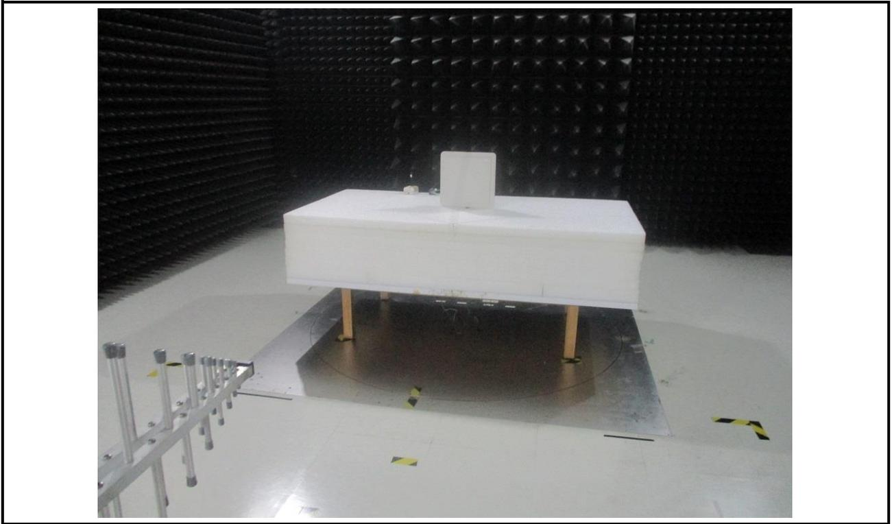
**Radiated Emission Above 1GHz Test**
