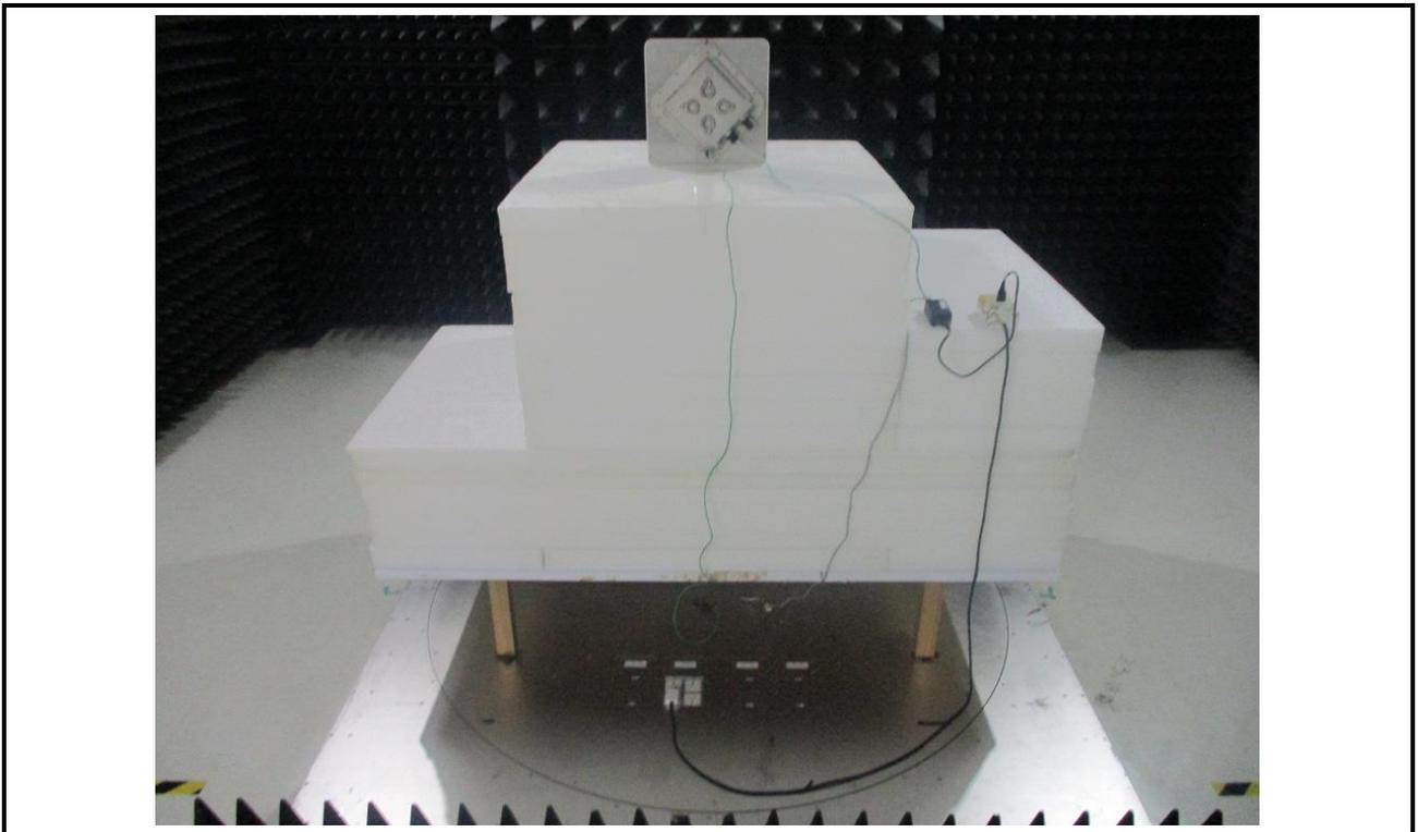
**Radiated Emission Above 1GHz Test**
