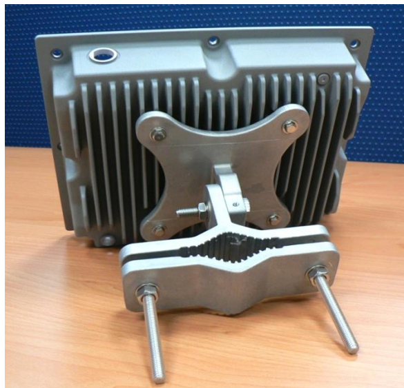
<Gemtek Small Cell Wall Mount Equipment Installation Example>
