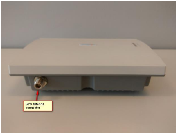
Figure 4: GNSS antenna port
