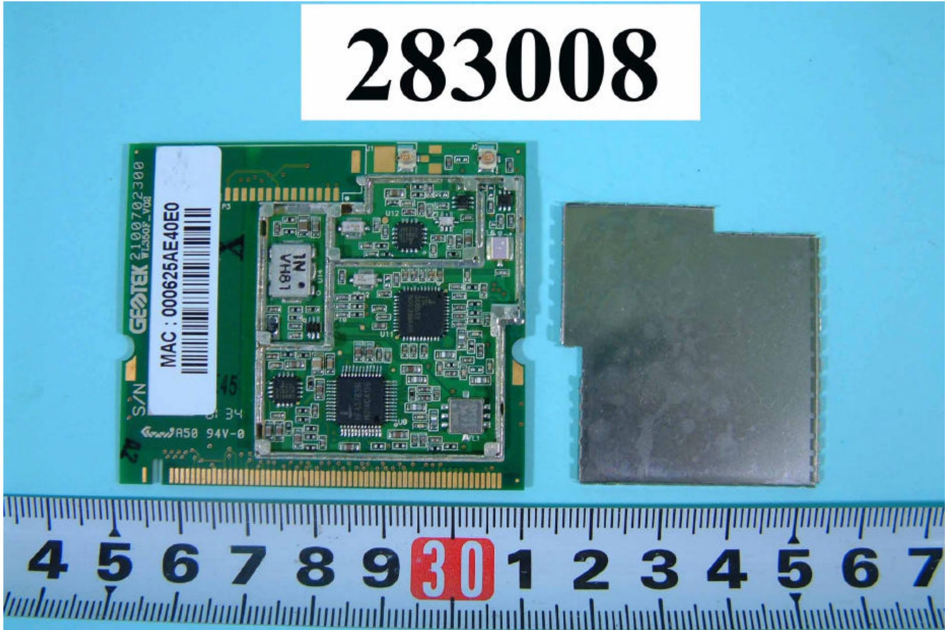
Front side of 11Mbps Wireless LAN Mini-PCI Card
