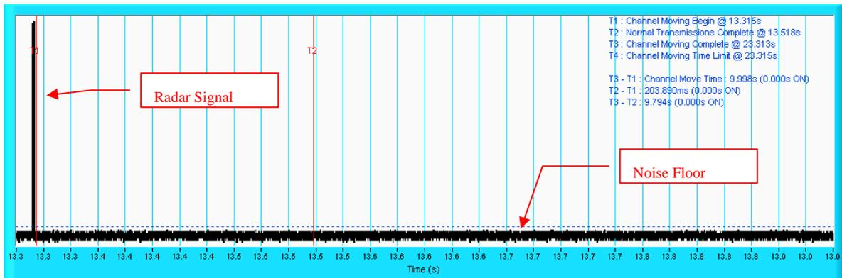
**NOTE:** An expanded plot for the device vacates the channel in the required 200ms.
