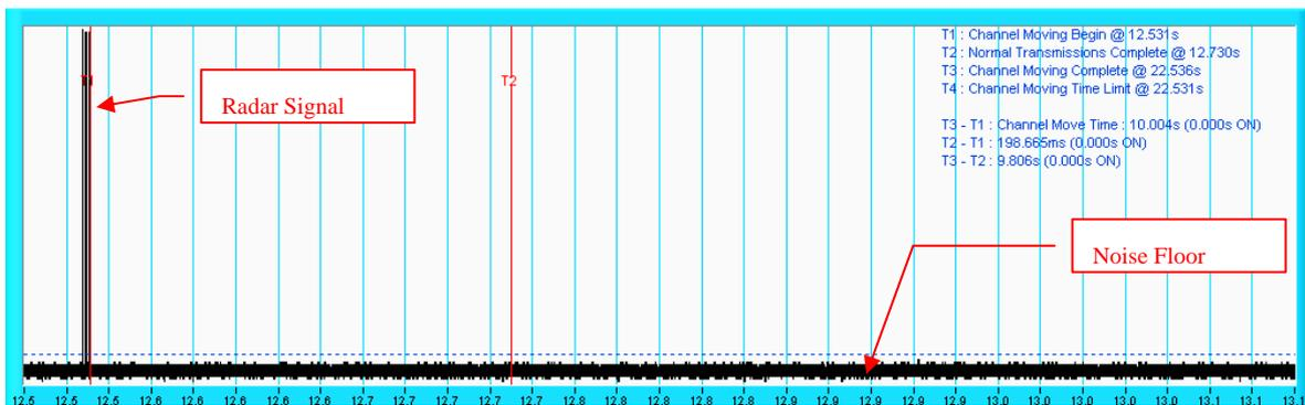
**NOTE:** An expanded plot for the device vacates the channel in the required 200ms.
