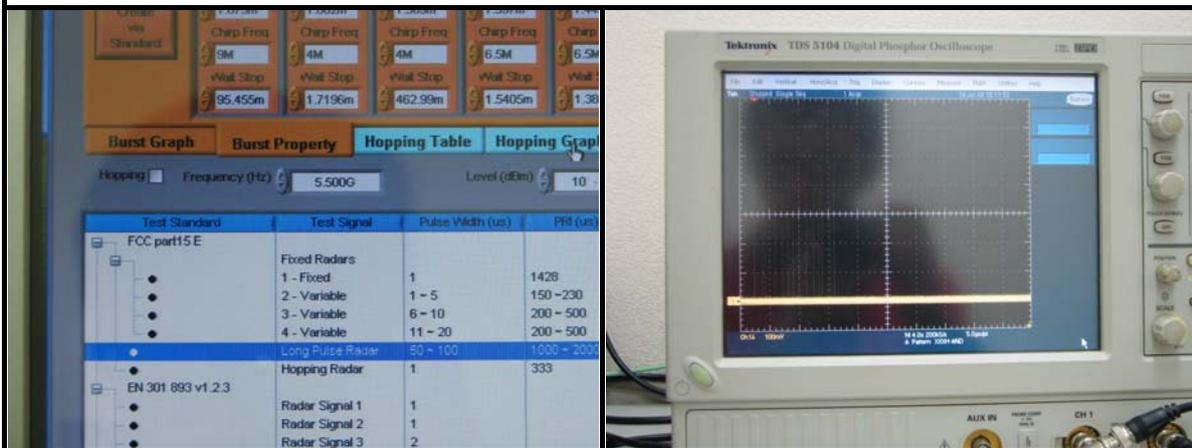
Radar 5 is used to test during DFS testing.
