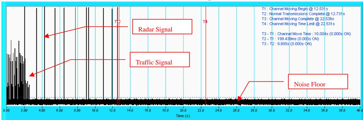
**NOTE:** T1 denotes the start of Channel Move Time upon the end of the last Radar burst. T2 denotes the data transmission time of 200ms from T1. T4 denotes the 10 second from T1 to observe the aggregate duration of transmissions.
