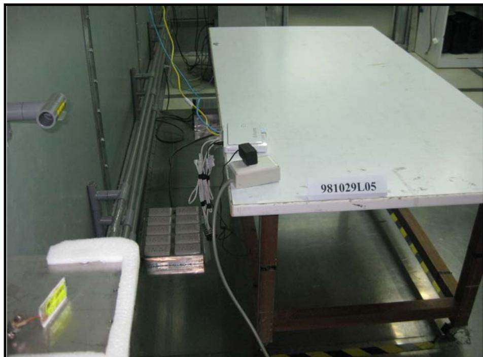
CONDUCTED EMISSION TEST (Test Mode B)
