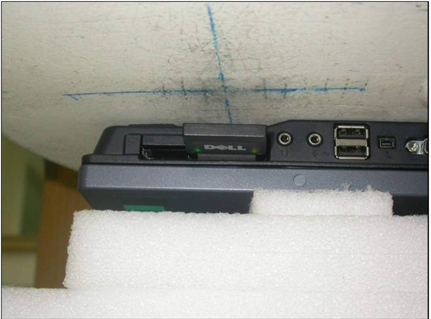
**The bottom of the EUT to the flat phantom distance 14 mm**
