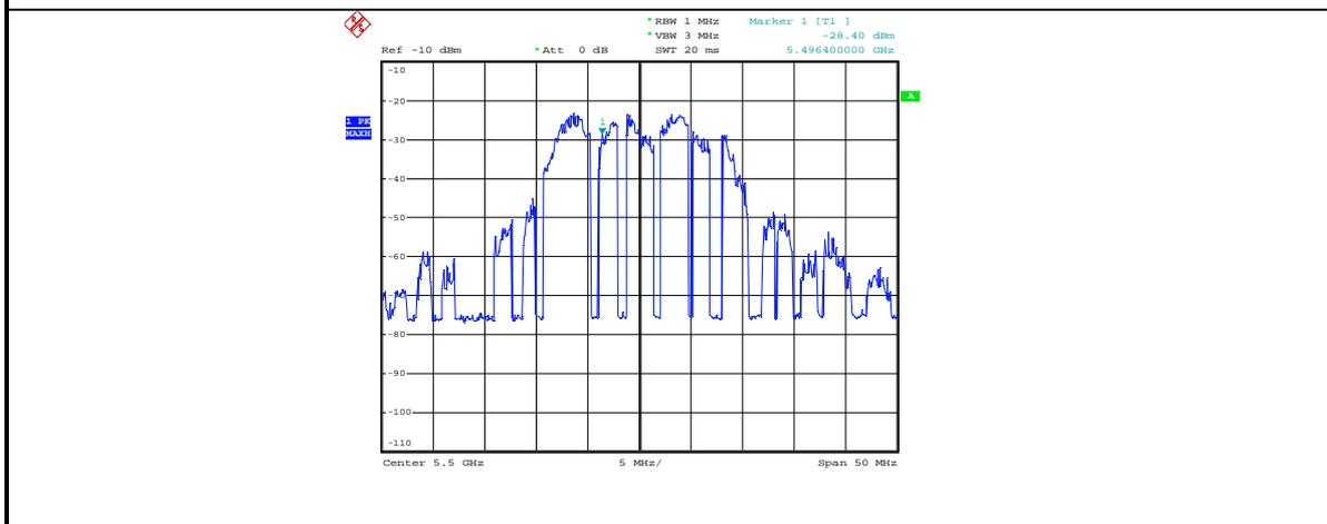
2) The client and DFS-certified master device are associated, and the movie can be streamed as specified in the DFS Order for a non-occupancy period test.
