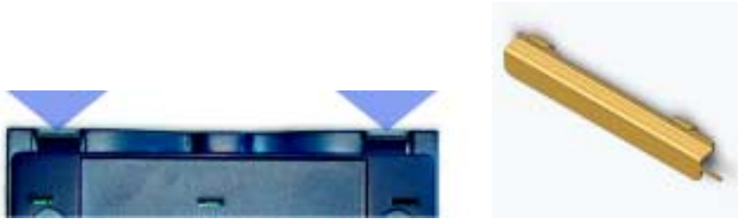
Figure 3 -- Removing the P-360 housing using the disassembling tool
