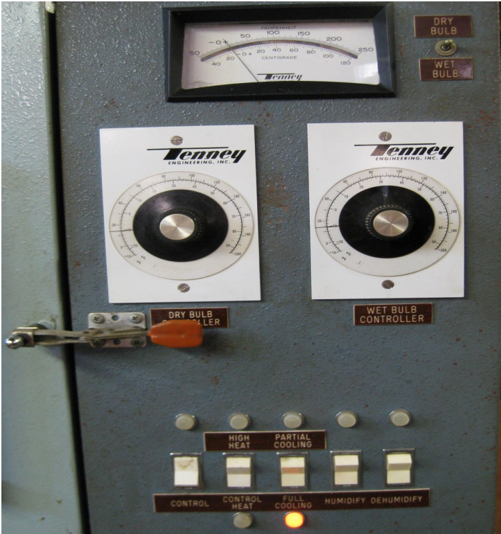
Photo 2 - Controls on Tenney Enviromental Chamber
