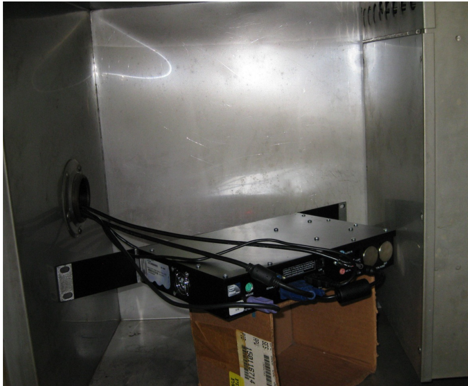
Photo 3 - CAP-DEC 1 placement inside Tenney Environmental chamber
