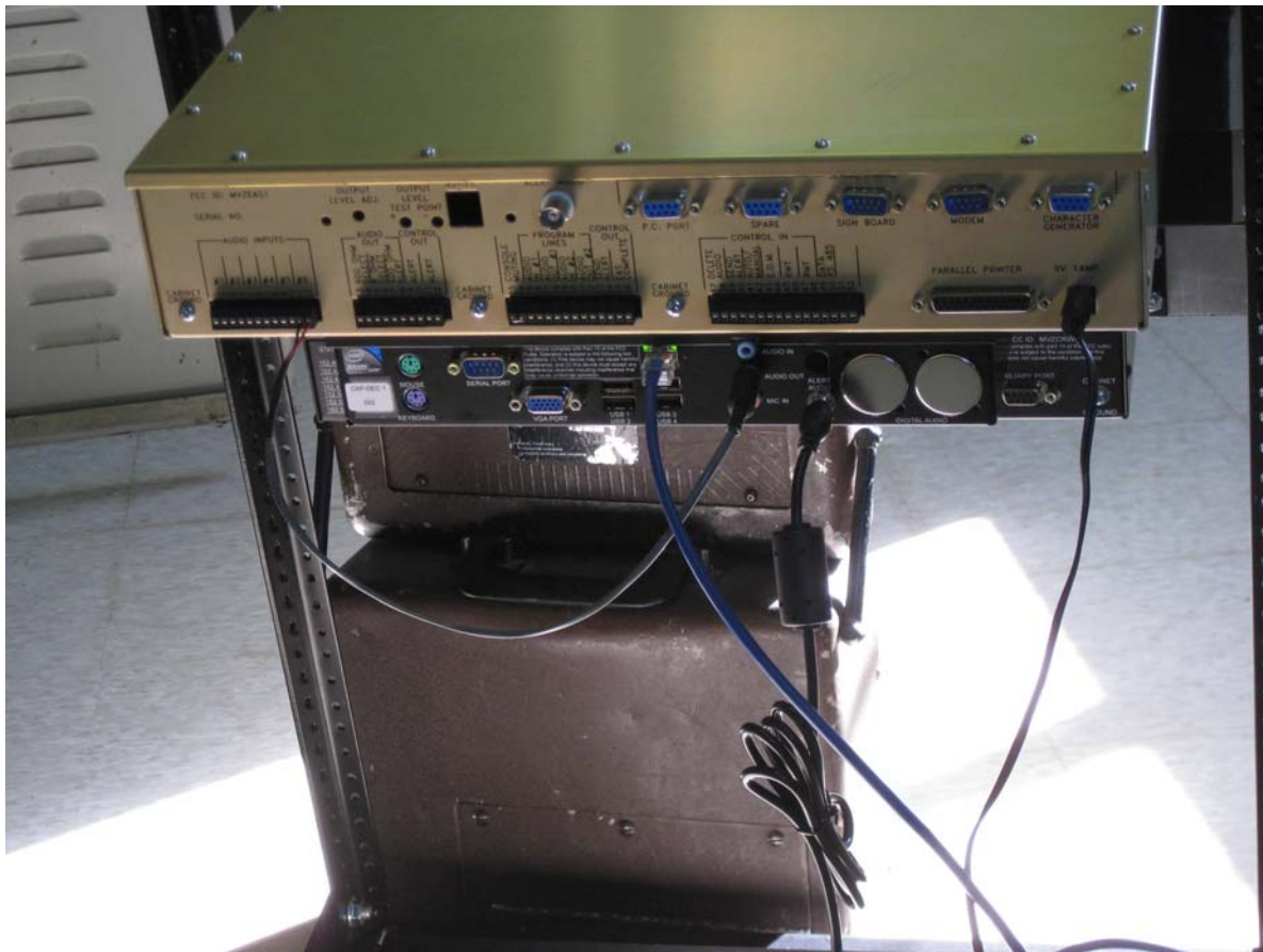
AM Test – AM RF Field Meter on Left (Rear View)
