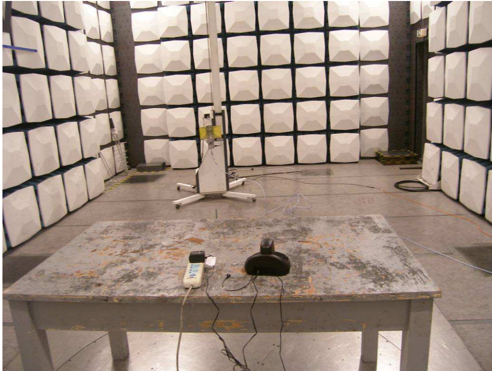
Photograph 4: Set-up for Conducted Emissions
