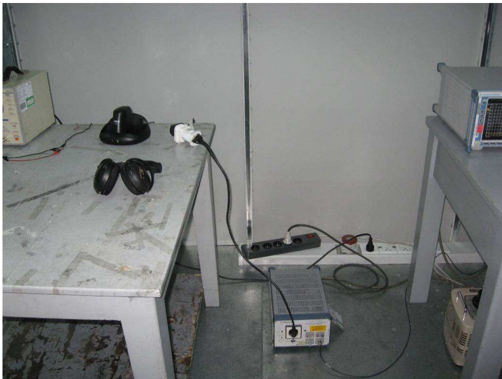
Photograph 4: Set-up for Conducted Emissions
