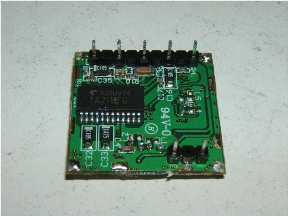
Internal View of EUT-7
