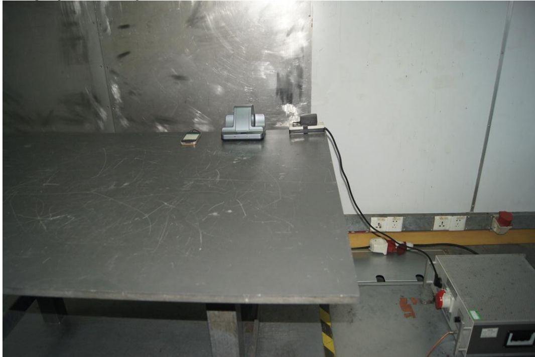
Photograph 2: Setup for Radiated Emissions below 1GHz
