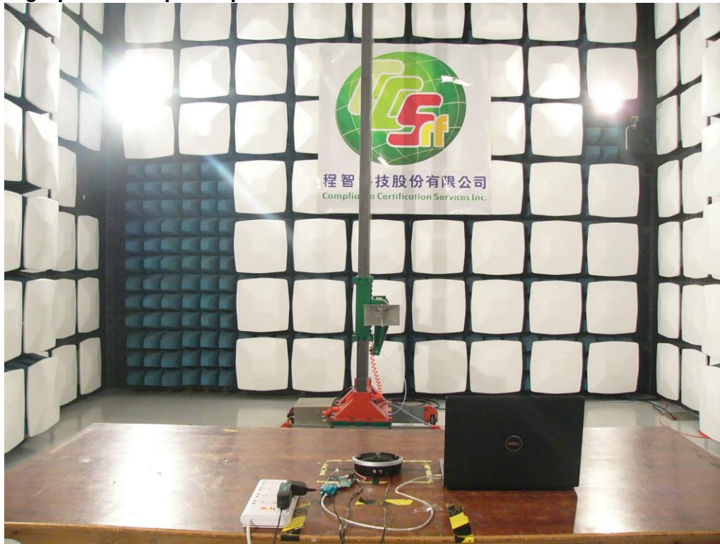
Photograph 6: Setup for Radio Spectrum testing
