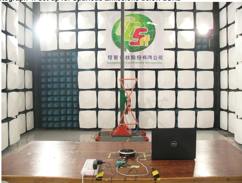
Photograph 4: Set-up for Spurious Emissions below 1GHz
