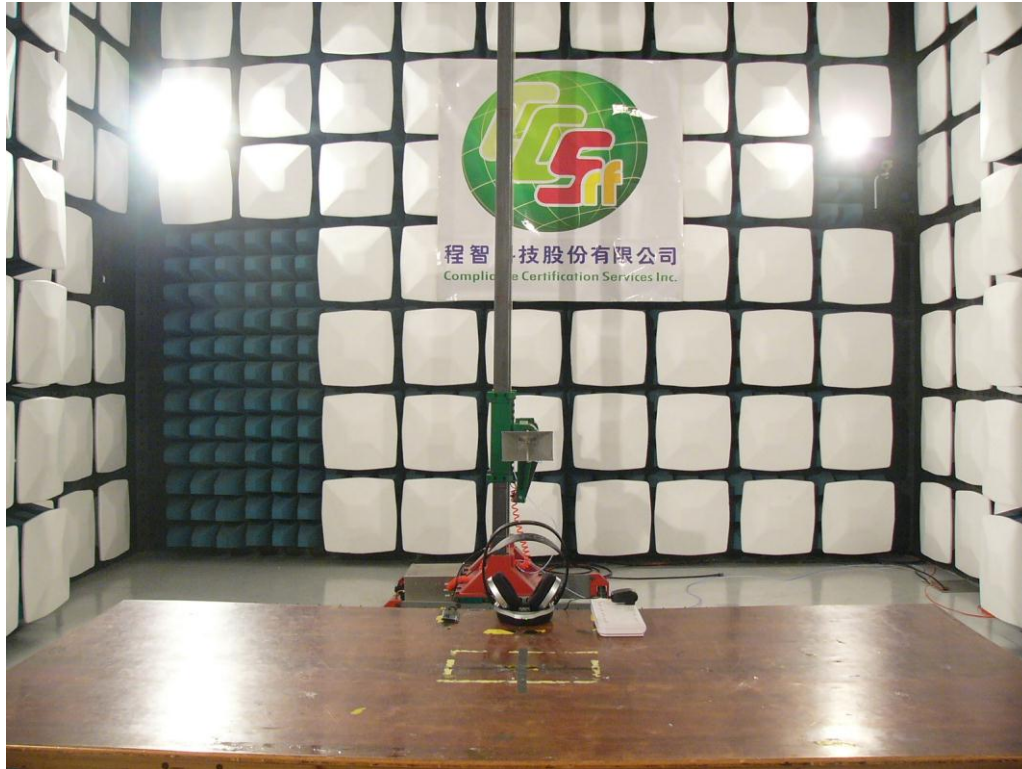
Photograph 4: Set-up for Spurious Emissions below 1GHz
