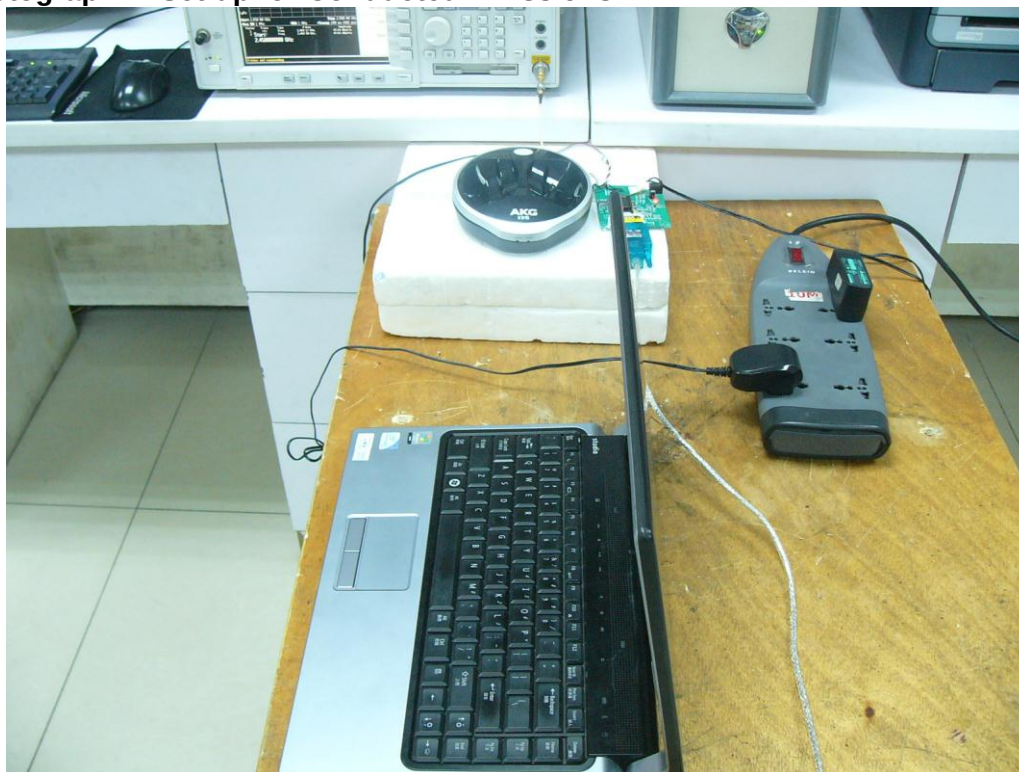
Photograph 2: Set-up for Radiated Emissions below 1GHz
