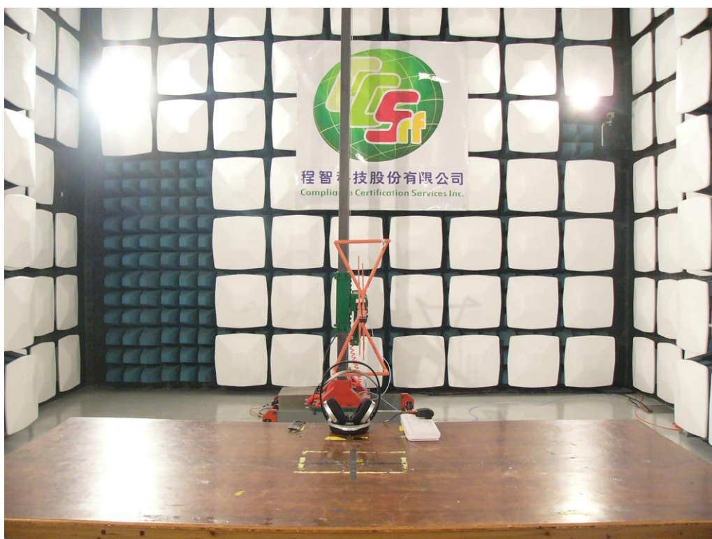
Photograph 2: Set-up for Radiated Emissions below 1GHz
