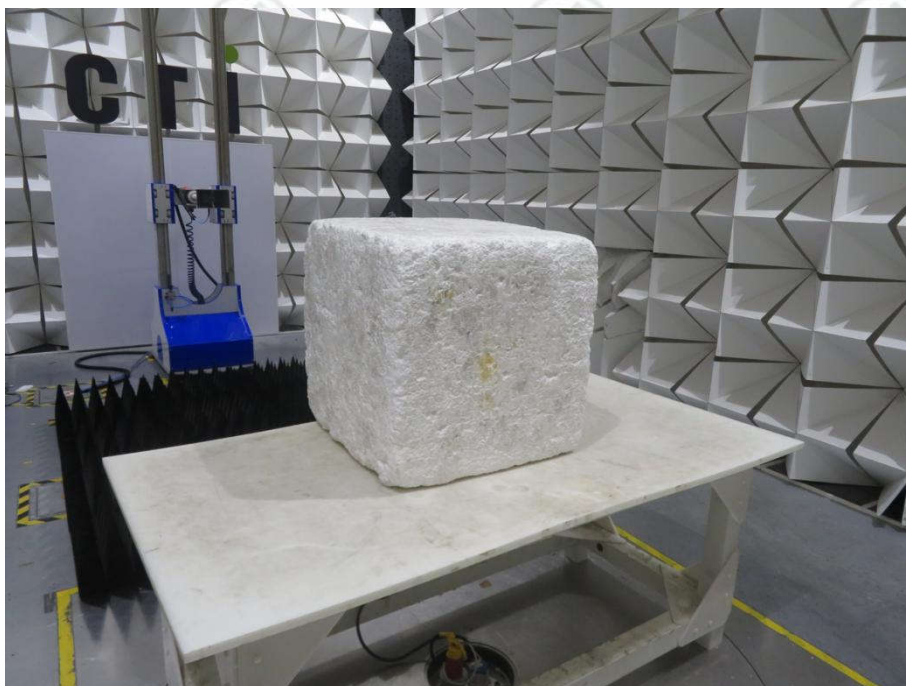
Radiated spurious emission Test Setup-3(Above 1GHz)
