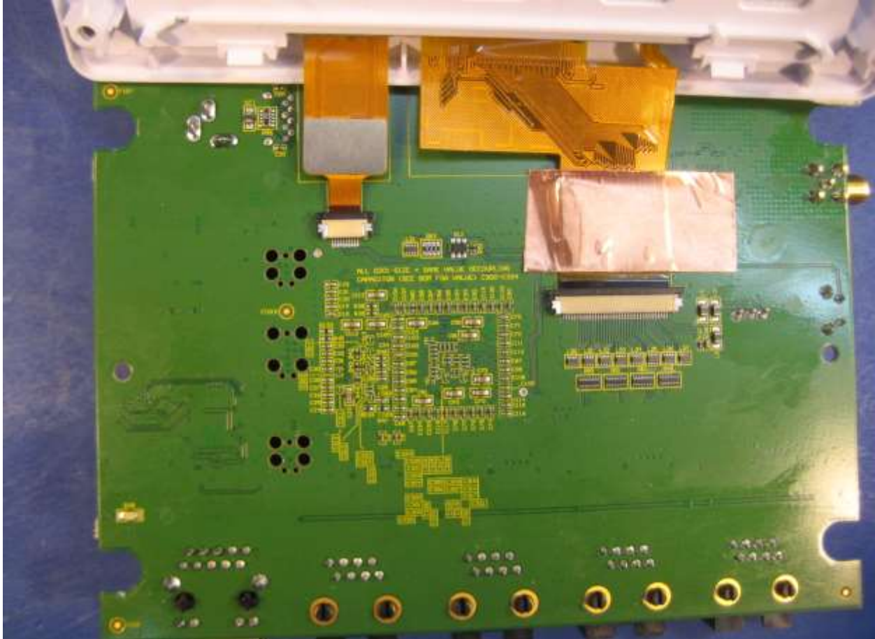
Mod 1 = Copper tape added to LCD display ribbon cable to suppress radiated emission below 1 GHz.
