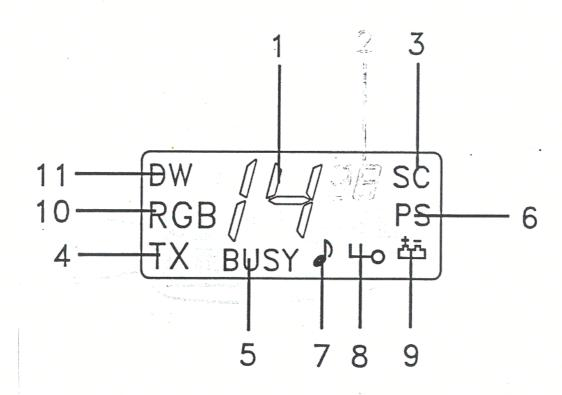
The KF-2100 is equipped with an LCD display to indicate its settings and functions. The Display incorporates automatic backlighting to allow it to be seen in the dark. Pressing any of the buttons except the PTT (Push-to-Talk) button, will illuminate the display. The display will remain lit for 5 seconds after any of these buttons is pressed.
