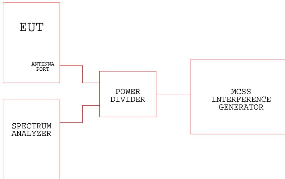
**Test Configuration Block Diagram**
