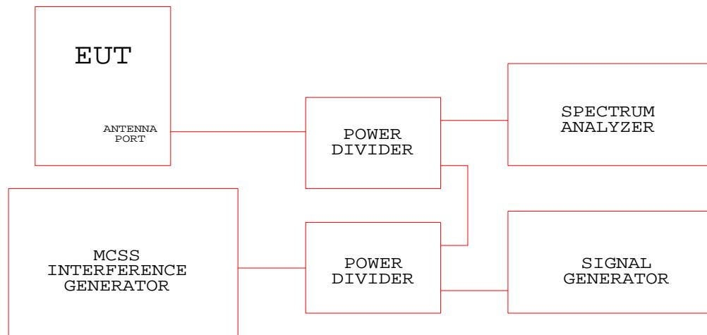
**Test Configuration Block Diagram**
