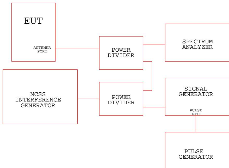
**Test Configuration Block Diagram
