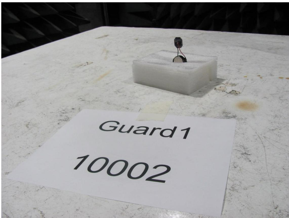
The EUT was placed on a foam block, in order to change the orientation
