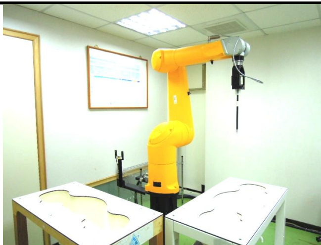
Fig-3.2 SPEAG DASY52 System
