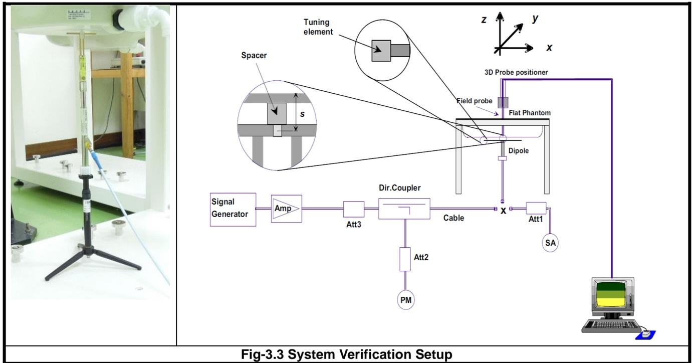
**Fig-3.3 System Verification Setup**
