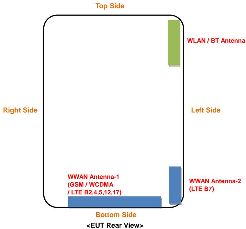
The separation distance for antenna to edge:
