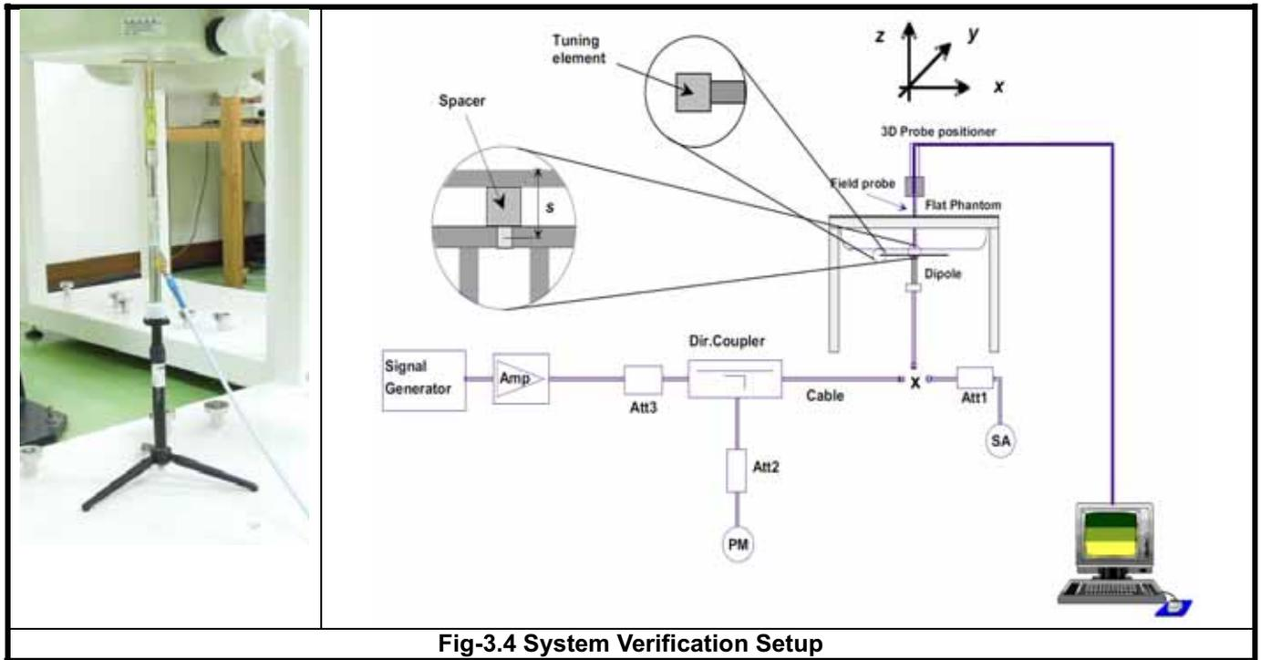
**Fig-3.4 System Verification Setup**
