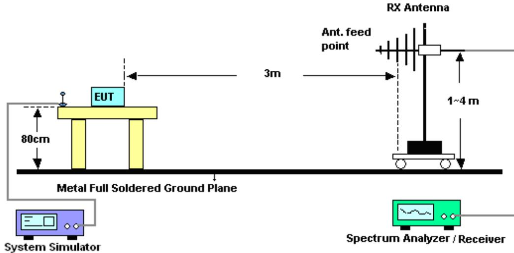
For radiated test above 1GHz
