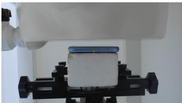
Front, Test Separation 10mm
