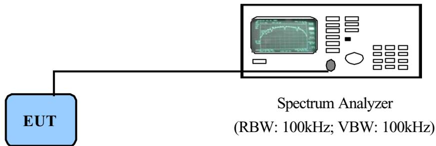
*P.S.: Notebook computer to control the EUT at maximal power output and channel Number and set antenna kit*
