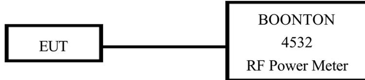
1. The output of the transmitter is connected to the BOONTON RF Power Meter.
