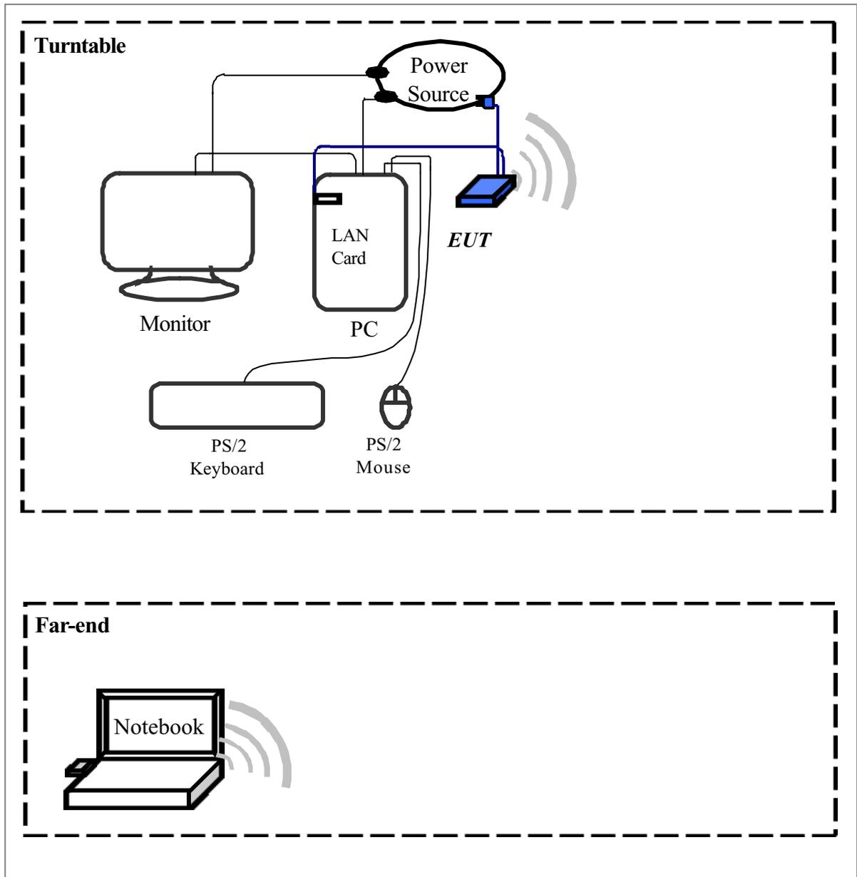
The tests below are carried with the EUT transmitter set at high power in TDD mode. The EUT is forced to select of output power level and channel number by computer.
