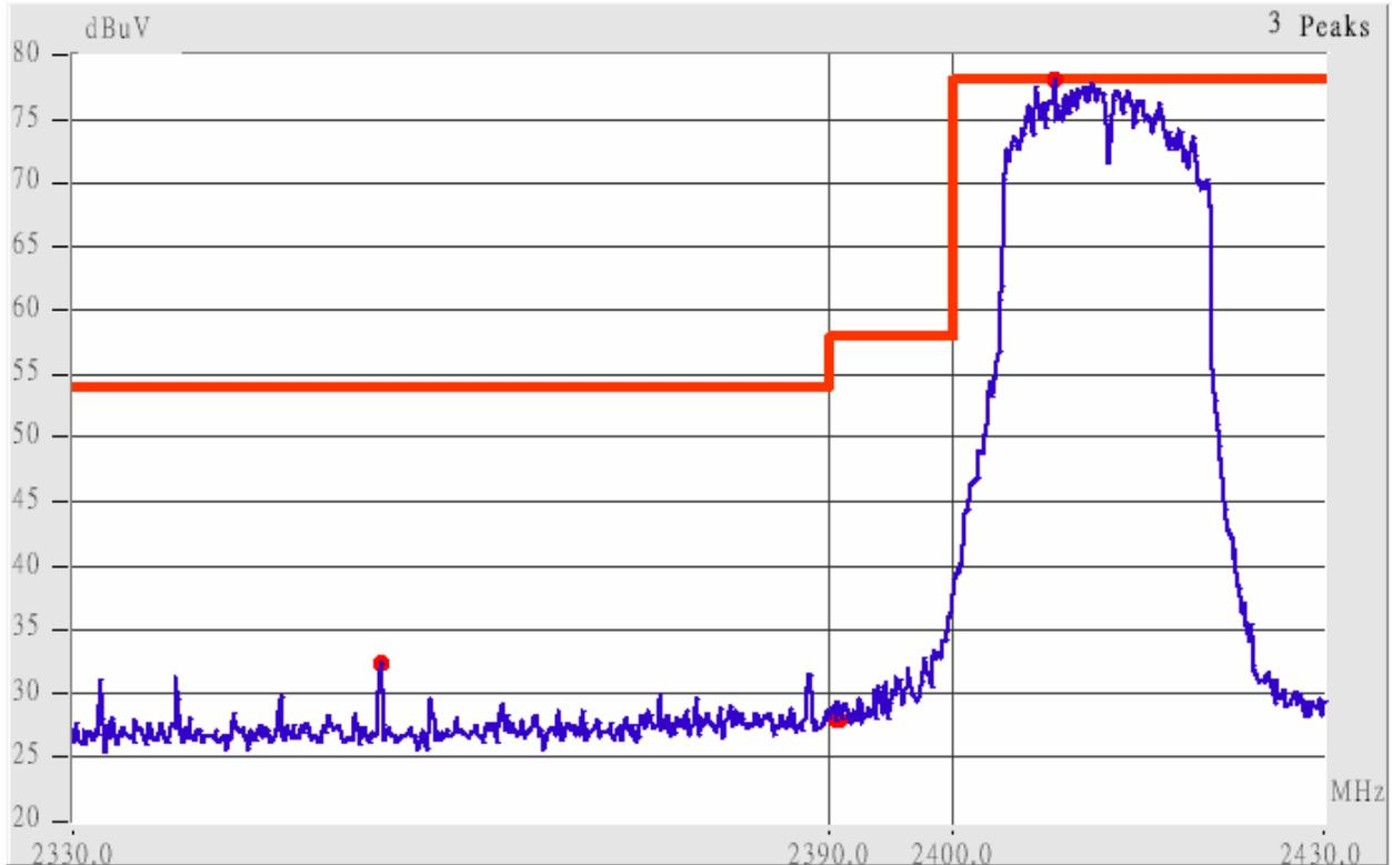
This is the hard copy of our bandedge measurement generated by our bandedge testing program. The plot shown above is the bandedge of channel 1.
