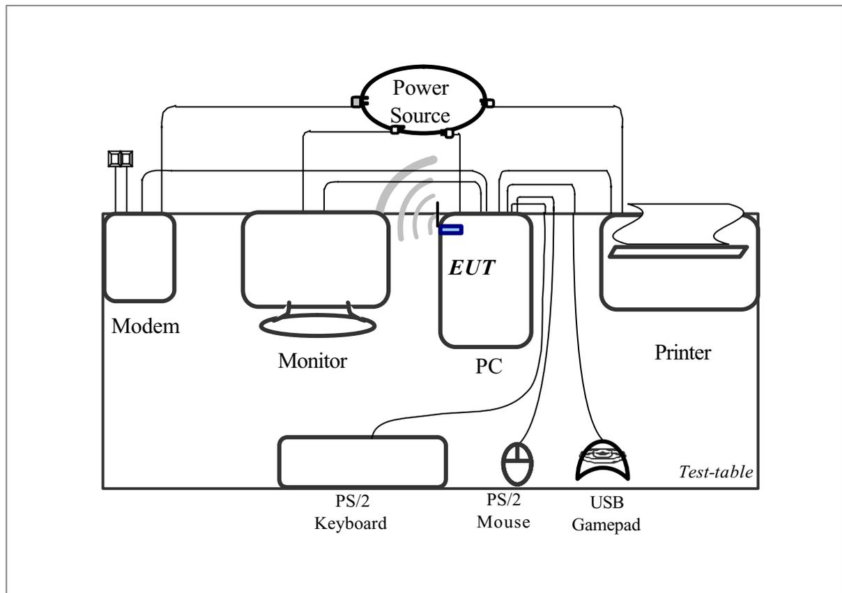
The tests below are carried with the EUT transmitter set at high power in TDD mode. The EUT is forced to select of output power level and channel number by PC.
